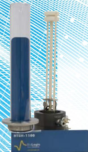
**High Temperature Sample Holder (HTSH-1100)** is a test fixture dedicated to characterization of electrical properties of solid materials using the parallel plate capacitor method over the temperature range between the room temperature and 1100 °C. HTSH-1100 can also be used for heat treatment in controlled atmospheres.
